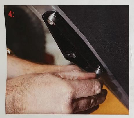
4: Install the brackets with the ball studs facing inwards using the stainless bolts and split washers provided.
