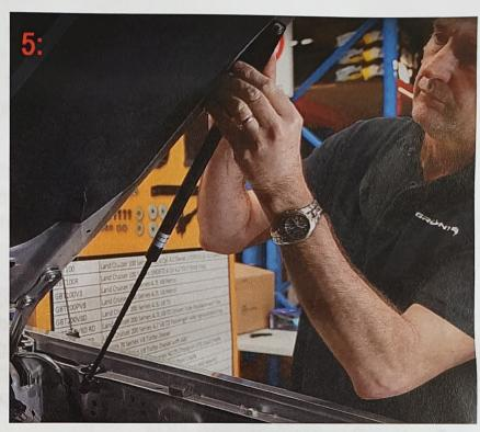
5: Last step is to push the gas struts onto the brackets as shown.
